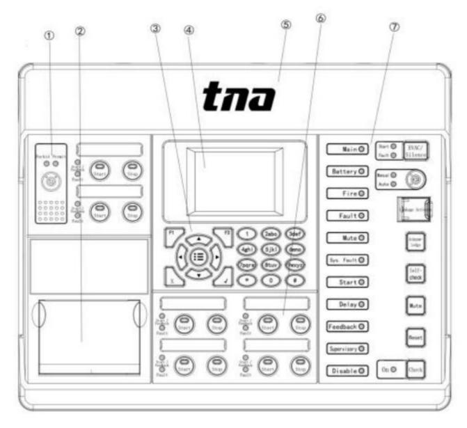
Diagram description: ①manual control switches ②printer ③key zone ④LCD display zone ⑤wiring cover ⑥manual control unit ⑦standard panel zone
